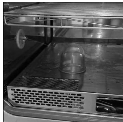
Fig. 4 Spraying the light disperser inside the climatic chamber
