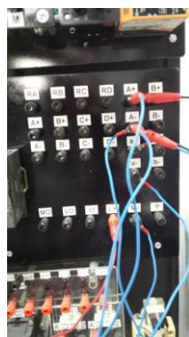
Fig. 12. Connect the conductors to the first application (with EM 231 RTD module)
