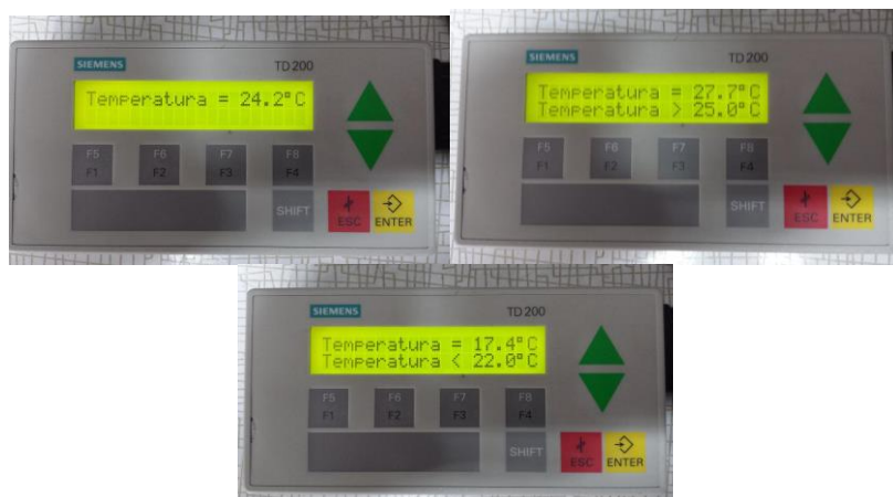
Fig. 13. Displaying the messages on the operator interface TD 200
