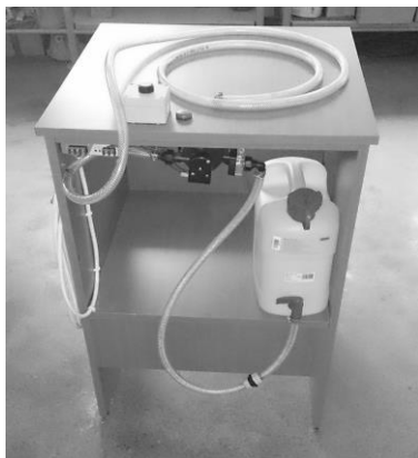
Fig. 3 Test rig for performing the thermal shock test
